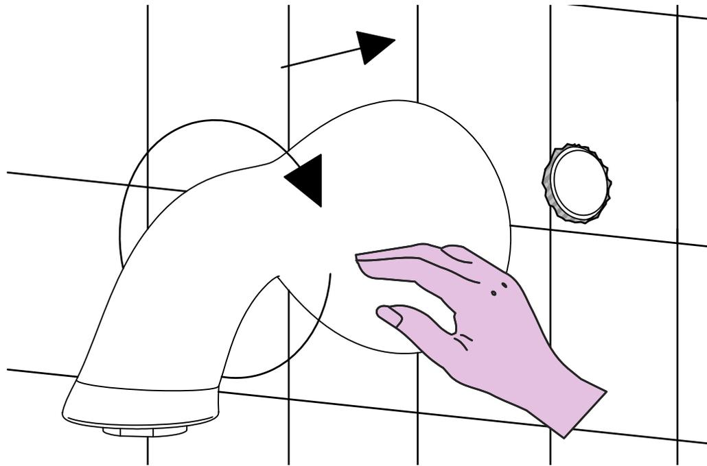
**SOSTITUZIONE AERATORE / AERATOR REPLACEMENT**
